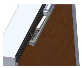
Place the arm on pull track roller and proceed with the tightening to end the arm mounting.
