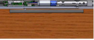
Manually pull arm and close the door to proceed with the next step "place it on pull track roller".
