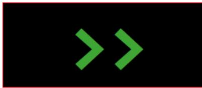
Green Static Arrow (Rest mode) Present personal security card to the reader mounted on the unit for authorisation.
